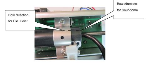
Align the level of silver plate and joint pipe.
