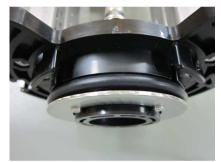
Insert the rubber bush into transducer part.
