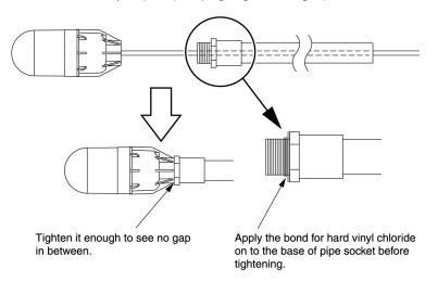
4. Fix the joint pipe and soundome with pipe guide (A).
