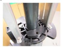
Rotate the plate 90 degree, lift it to split into 2 pieces.
