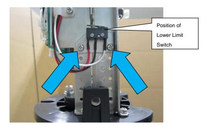
Remove 2pcs screws shown above to lower the lower limit switch for longer stroke.
