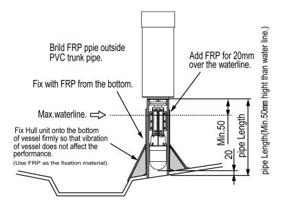
Add the extruding part of approx.5mm with FRP for the purpose of reducing the water pressure inside the trunk pipe while sailing.
