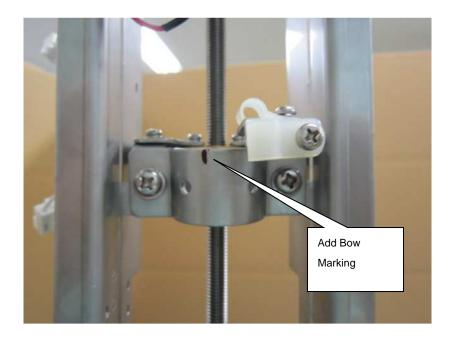
After fixing the location of electric hoist, put the marking with pen on the hoist and trunk pipe.
