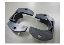
Rotate the cut area of each layer for 120 degree and insert 4 layers to the joint area.
