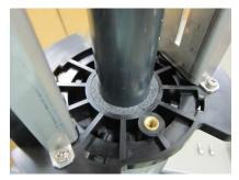
Lastly, tighten the plate with M6x20 screws and flat washers.
