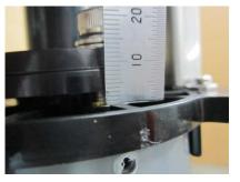
Add some water for smoothing O-ring and trunk pipe. Insert the joint pipe into trunk pipe carefully without causing any damage onto soundome. Keep pushing the joint pipe until the location of trunk pipe reaches the fixation position.
