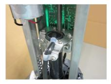
Place the PCB back to the original location and fix it with 6 screws.
