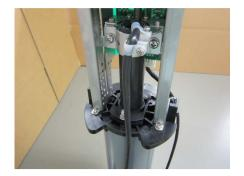
PCB side has the connection between power and Upper/Lower signal lines. The opposite side has the transducer cable.
