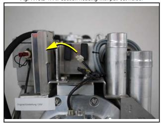
2. Tip the two fasteners 90°.
