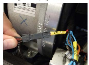
Fig. 12.5-1: Not Stop bridge in the cable harness
