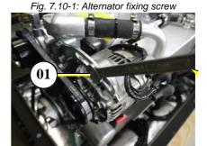
Fig. 7.10-2: Alternator fixing screw
