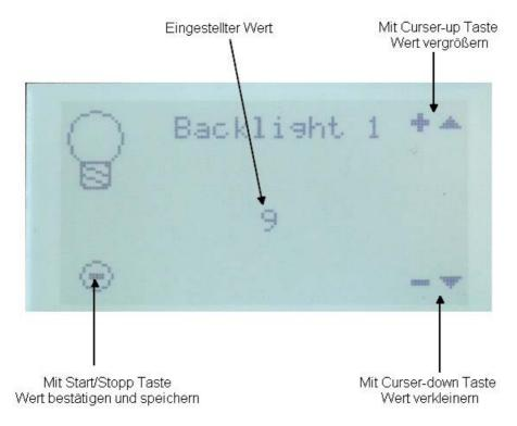
In the sub-menus, set the desired values with the cursor Note: buttons, and then confirm your settings with the Start/ Stop button.
