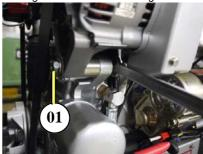
Fig. 7.10-3: Replacing the V-belt
