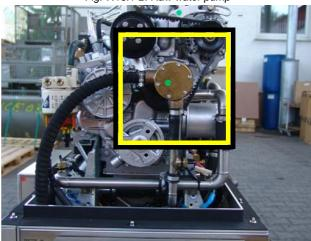
Remove the cover of the raw water pump by loosen the screws from the housing.
