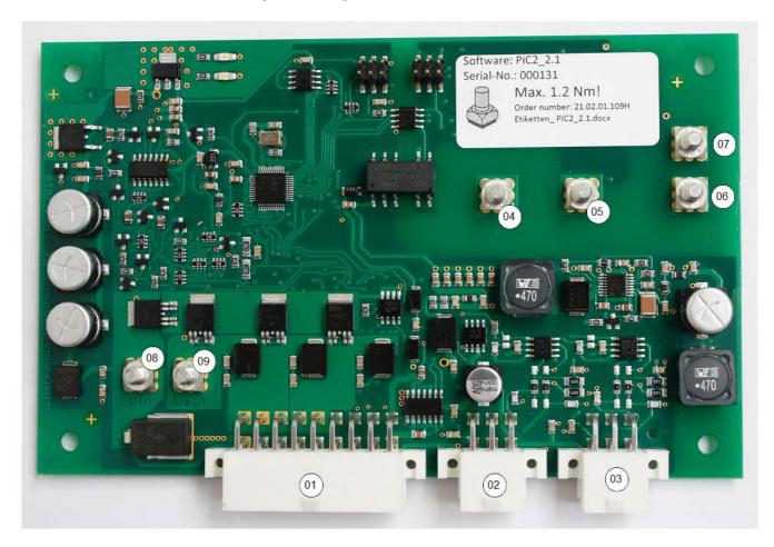
The Panda iControl2 controller is connected to the wire harness with the 18-pin jack. The centre 6-pin jack is designed for the Fischer Panda standard bus. The Panda iControl2 panel is connected to this jack. The Fischer Panda CAN bus is connected to the 6-pin jack at the bottom right of the circuit board. The configuration of the connectors is given in the subsequent tables. Siehe "Terminal assignments on the Panda iControl2 controller" auf Seite 156.
