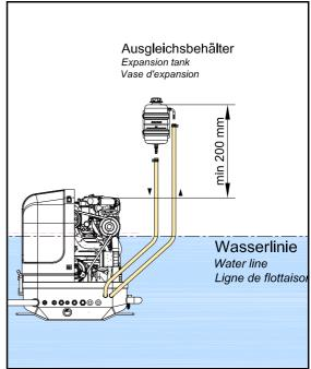
The external cooling water expansion tank may be filled only up to the lower edge of the lower tension tape (see note "max") in the maximum filling level in cold condition.
