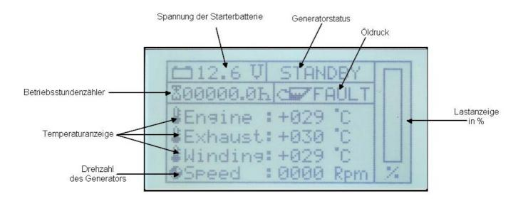
The Display shows the iControl board input voltage.
