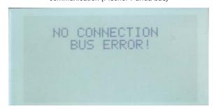
If the communication connection is lost, the generator shall be secured (open battery disconnect switches), and all plug-in connections and cables shall be checked for firm seating or damage.
