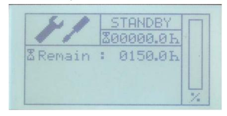
The total operating hours of the generator are given on the default display screen and on the service information screen. By actuating the cursor-up and cursor-down button in stand-by mode, the service screen can be accessed. This screen is marked with a screwdriver/spanner symbol. Here, the time until the next service is given. By actuating the cursor-up or cursor-down button, you can return to the default screen.
