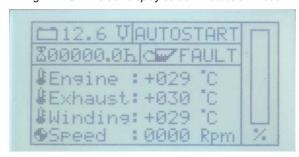
The autostart function will remain active even after the controller is switched off and on again with the On/Off button. To deactivate the autostart function, the flag in the EEPROM must be reset with "Disable" as described above.
