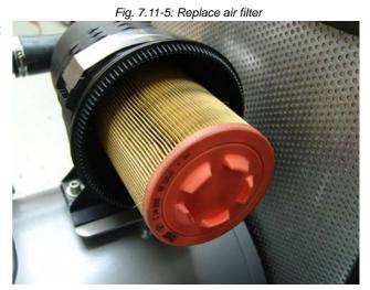
7. Blow out filter insert in folding direction maximum pressure: 5 bar.
