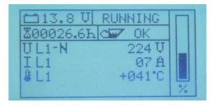
This screen provides the latest inverter output voltage of the single phases with the matching conductor current and the circuit board temperature. The inverter will be switched off at a circuit board temperature of 75 °C. You can access the inverter screen by actuating the cursor-up button while in operation mode.
