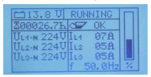
This screen provides the latest inverter phase voltages. You can access the inverter screen by actuating the cursor-up button while in operation mode.
