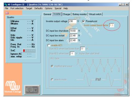
Fig. 10.6.2-1: Settings in the Victron VE configure II Software
