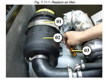
Fig. 7.11-2: Replace air filter
