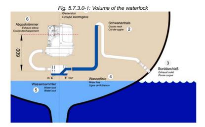
If there are any doubts, a verification can easily be made by temporarily using a clear-sighted hose (1) as exhaust hose. In that way, the cooling water level can be checked very easily.
