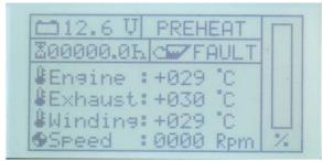
After pre-heating, the starter is initiated, accompanied by the text output "STARTING" in the status field of the default display screen.
