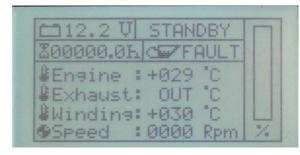
Fault: "Winding", winding temperature too high
