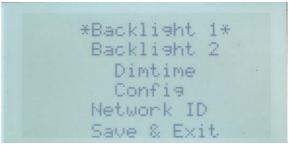
The Start/Stop button is used for confirming a selection in the set-up menu. If you confirm the row marked with the \* with the Start/Stop button, you will access the selected sub-menu.
