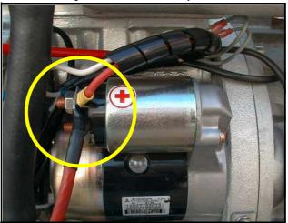
Fig. 5.11.2-2: Negative Battery Cable
