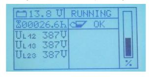
This screen provides the latest inverter output voltage of the single phases with the matching conductor current and the circuit board temperature. The inverter will be switched off at a circuit board temperature of 75 °C. You can access the inverter screen by actuating the cursor-up button while in operation mode.
