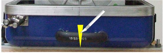
The rubber hose for the external vent valve will be cut...
