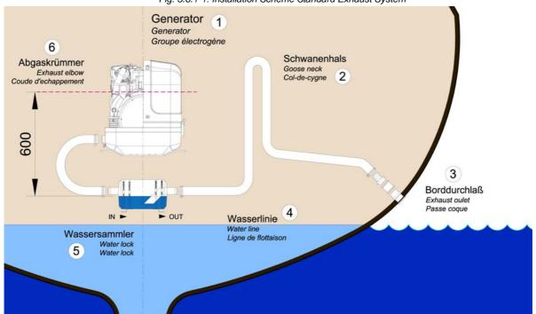
Fig. 5.6.1-1: Installation Scheme Standard Exhaust System
