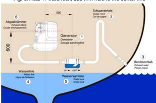
Fig. 5.7.3.2-1: waterlock, 500 mm next to the center line
